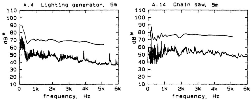
Figure 2 Examples of background noise spectra and predicted masked thresholds.
