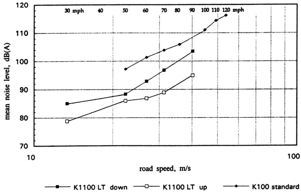
Figure 3 Noise levels measured under Helmet 21 during road trials on the K 1100 LT motorcycle with windscreen down and up, and on the K 100 motorcycle with standard windscreen height.
