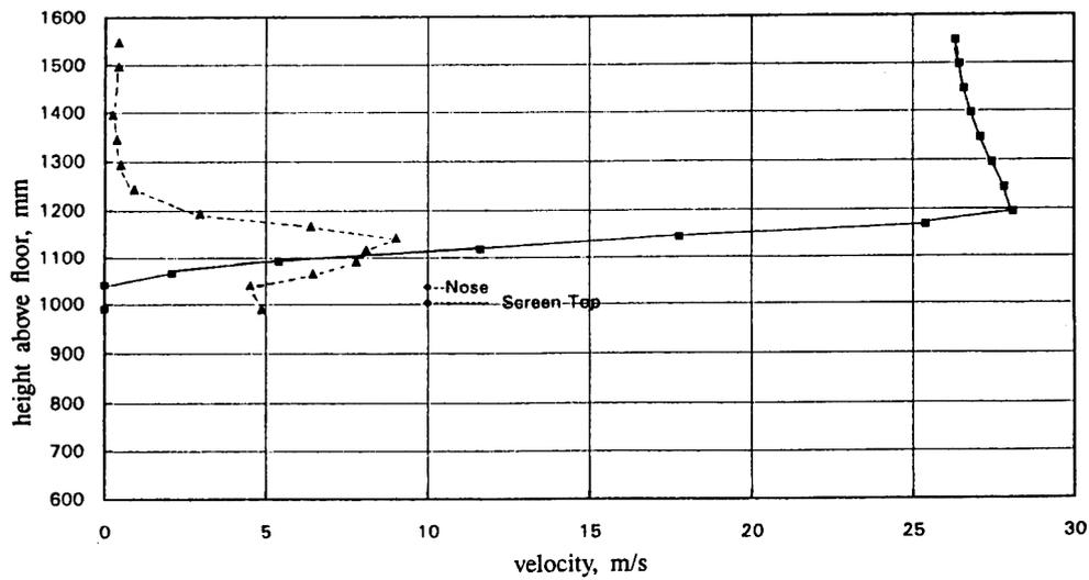
Figure 2 Results of pilot static tube and hot wire anemometer traverses on the K 100 motorcycle with standard windscreen. Squares show the mean velocity parallel to the tunnel length. Triangles show the rms velocity fluctuations x 2. The heights of the windscreen and rider's nose are also shown.
