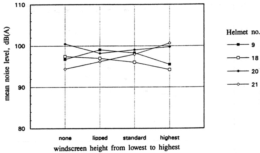
Figure 1 Variation of noise levels with windscreen height at 27 m/s nominal air speed.
