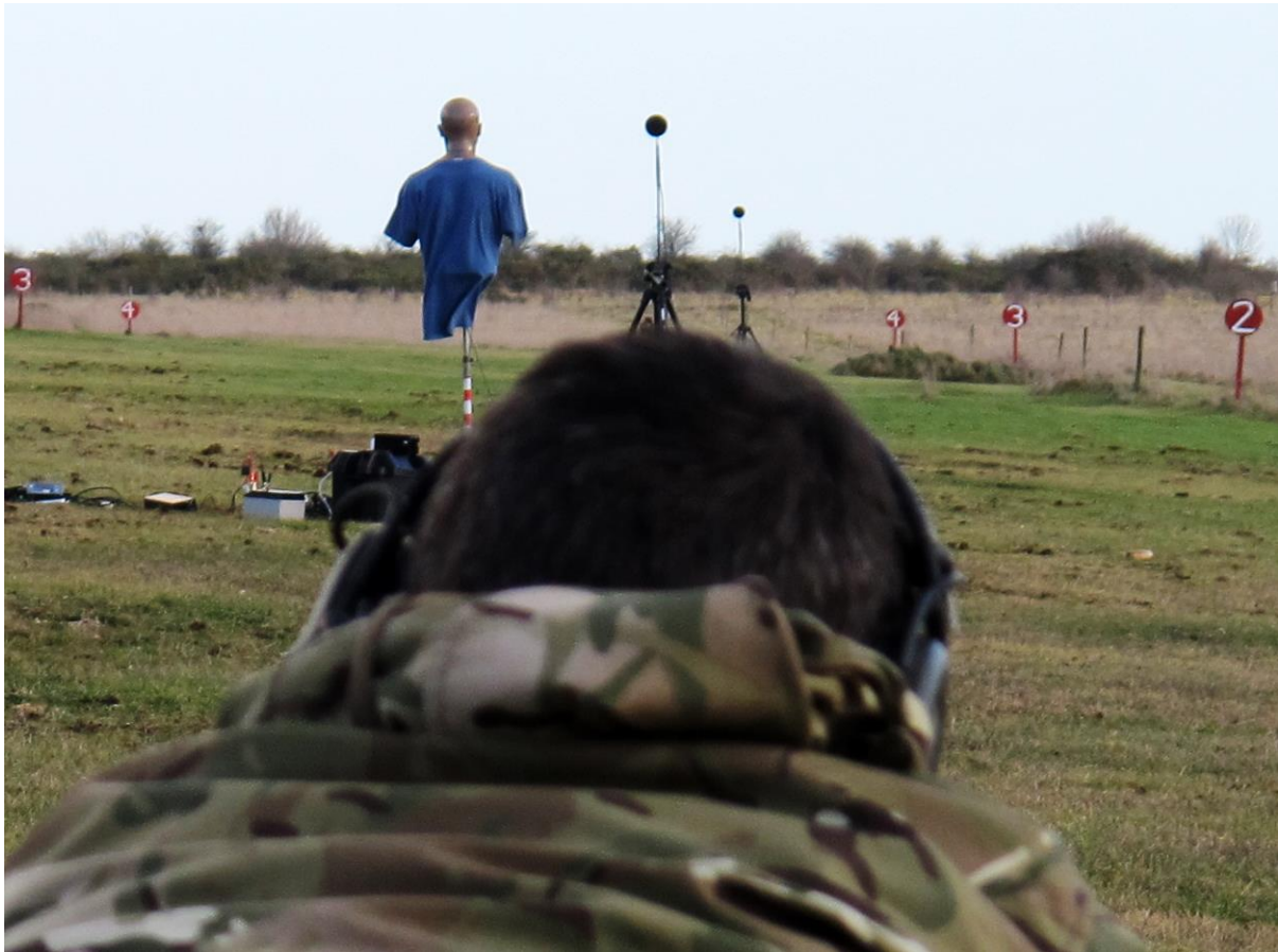
Fig. 3. Firer's view of the Kemar manikin with the quarter-inch microphone to the right.
