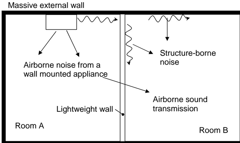
Figure 1 Schematic of the structure borne noise problem
