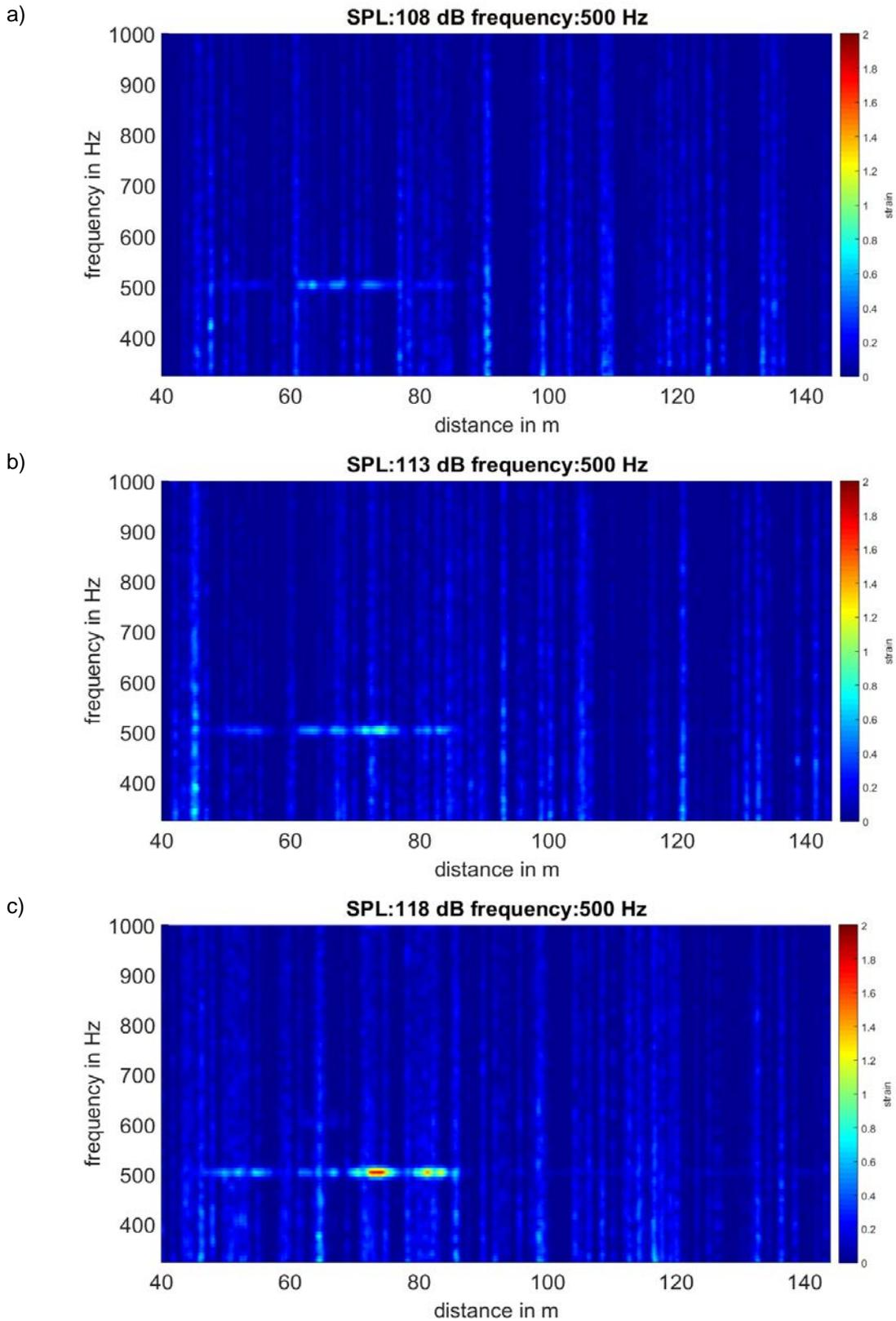
Figure 2. Measured pressure induced strain in the reverberation chamber for 500Hz excitation and different sound pressure levels a)108dB, b)113dB, c) 118dB
