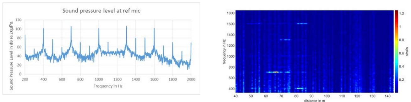
Figure 4. Multi-tone signal applied SPL at reference microphone 1cm from the fibre (left plot), strain colour map distance vs. frequency (right plot)
