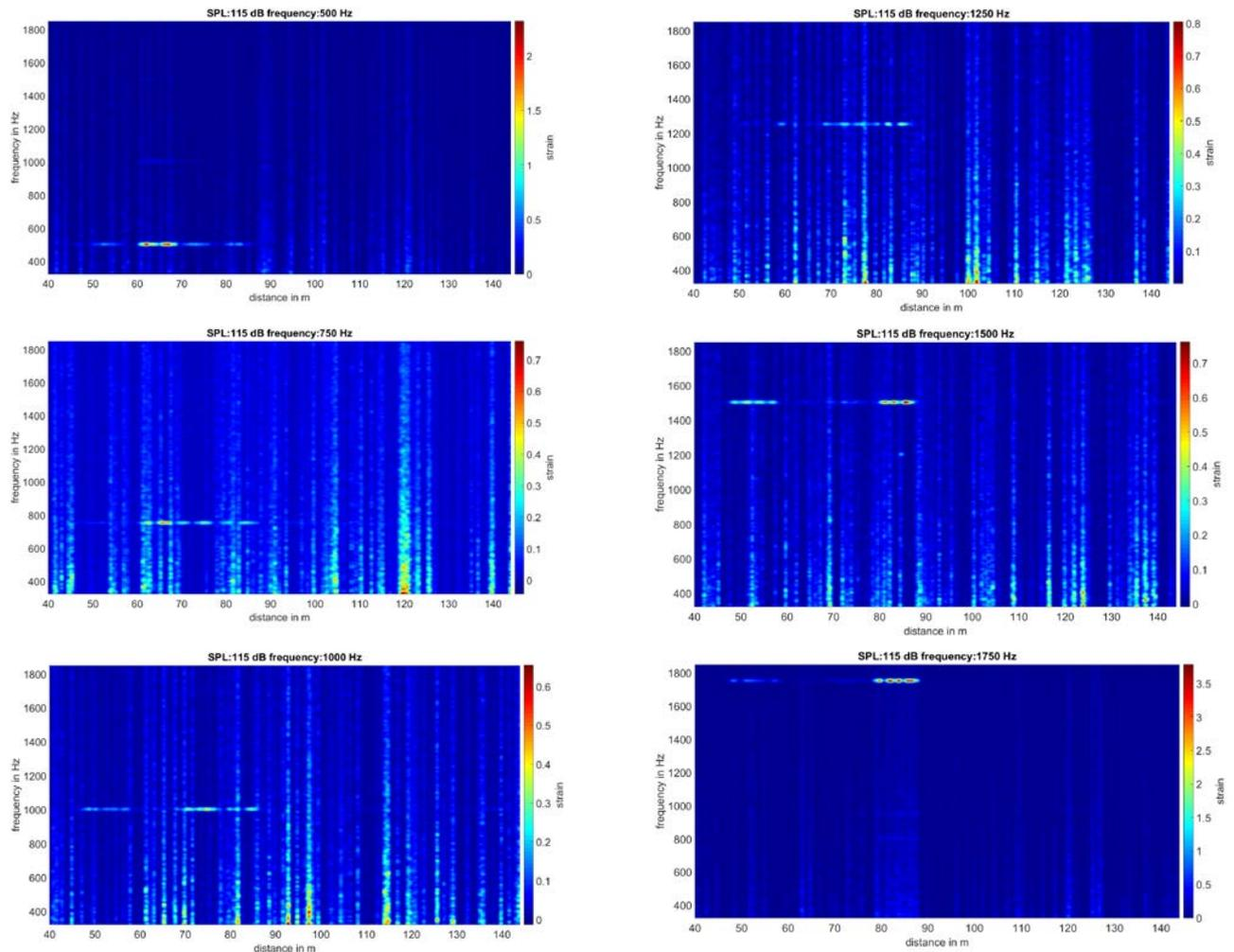
Figure 3. Measured pressure induced strain in the reverberation chamber for 115dB SPL for single tone excitations from 500 to 1750Hz with 250Hz step excitation, note that scale is not normalized and is different for each plot
